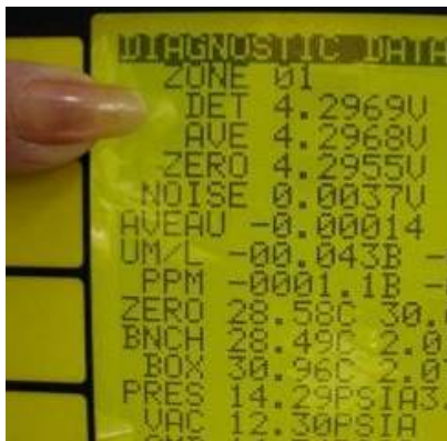
Figure 7. Detector voltage should be between 4.2 and 4.3 VDC
