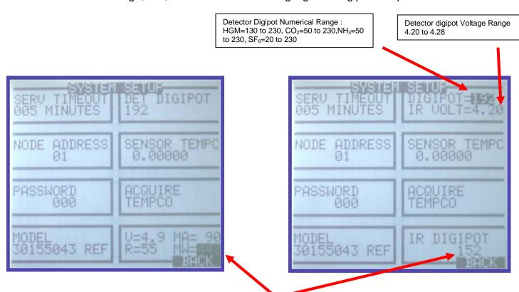
NOTE - Go into IR DIGIPOT and check the MW setting. These are guidelines and typical MW settings but this setting will <u>not</u> cause a FAULT. Any value as needed in here is acceptable.
