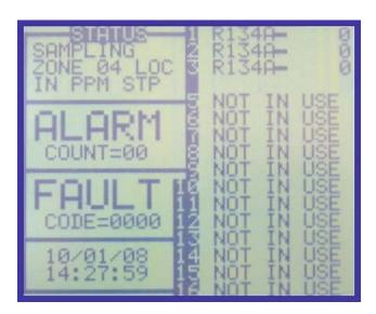
To correct for codes 200, 2000, 4000 and 8000 – from the front screen on the MZ select the top left block (under STATUS) and press enter. This will take you to the SETUP screen.
