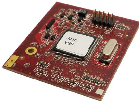
Figure 2. Microprocessor Module Removed from the RD's Main Board
