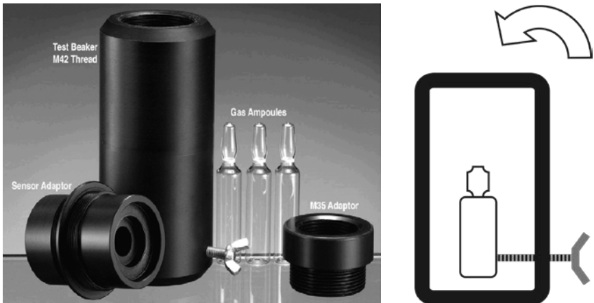
Figure 9. Gas Ampoules for Bump Testing
